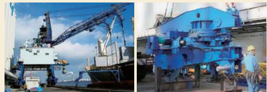
Left: Unloaders discharge 600,000 tons of wheat in annual capacity to storage silos from ships. Right: The seismic isolation systems
