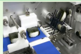
Seaweed wrapping unit for onigiri rice balls
